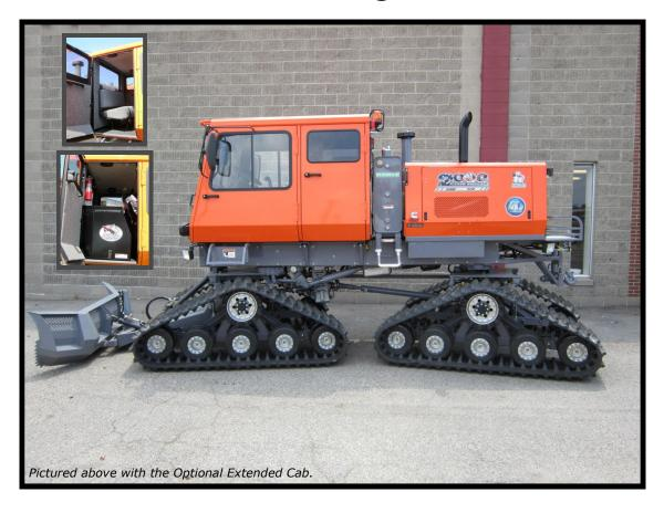
ENGINE...... 6.7 Liter 6-Cyl Tier 4i Cummins 173 HP
