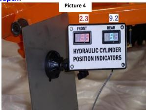
What the Hydraulic Cylinder Digital Position Indicators shows the operator, is a "number" that equals "a cylinder position" that is always repeatable!
