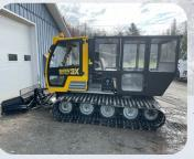
Thanks to the new passenger cabin, R.O.P.S. certified, the Snow Rabbit safely and efficiently transports up to 6 passengers to the desired location. It
